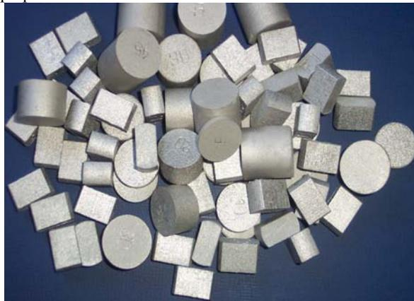
Fig.6. Ni-Cr dental alloy pellets
