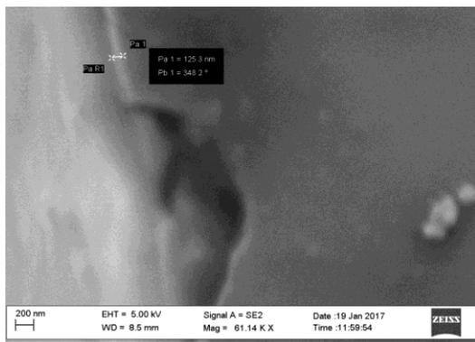
Fig. 7. Film thickness
