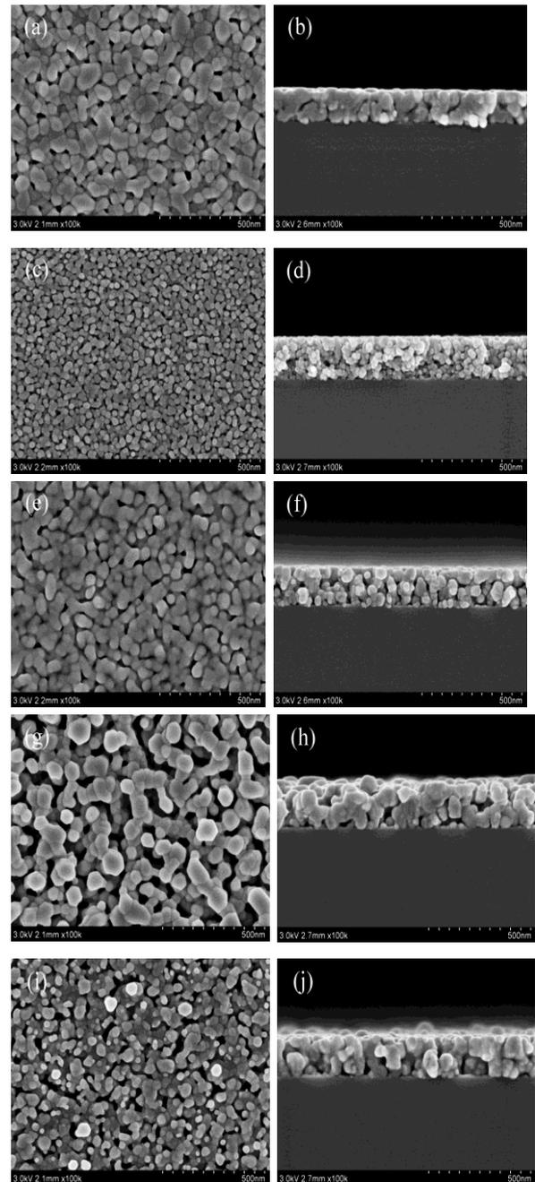
Fig. 2. Surface and section morphology images of the pure ZnO thin film (a, b), and Sr-doped ZnO thin films annealed at 400 °C (c, d), 450 °C (e, f), 500 °C (g, h) and 550 °C (i, j)
