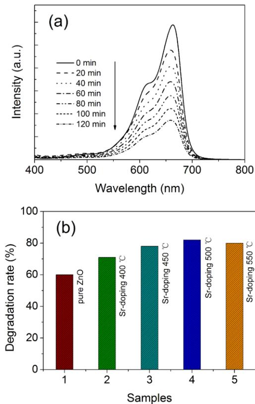
Fig. 5. The absorption spectra of MB solution at different reaction time (a) and degradation rates of the ZnO thin films (b)
