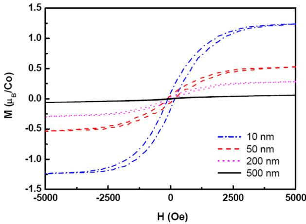
Fig. 3. Magnetization hysteresis curves of  $\text{Zn}_{0.95}\text{Co}_{0.05}\text{O}$  films with different thicknesses deposited under  $p_{\text{O}_2} = 0.075$  Pa and  $T_s = 450$  °C measured at room temperature.
