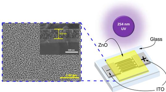
Fig. 1. FESEM image of ZnO thin film and schematic diagram of the device under UV radiation (color online)
