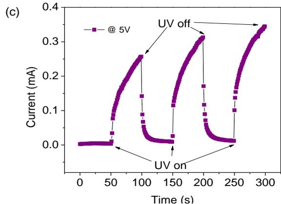
Fig. 3. Current-time characteristics of the device in the (a) dark and (b) UV-illuminated condition, and (c) time-resolved UV photocurrent on/off plot of the device biased at 5V (color online)
