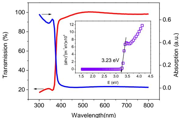
Fig. 2. Optical transmission and absorption spectrum of the ZnO thin film. Insert is the Tauc plot (color online)
