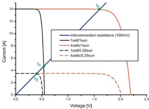
Fig. 4. Calculated I-V plot for multicrystalline solar cell and module assumption.
