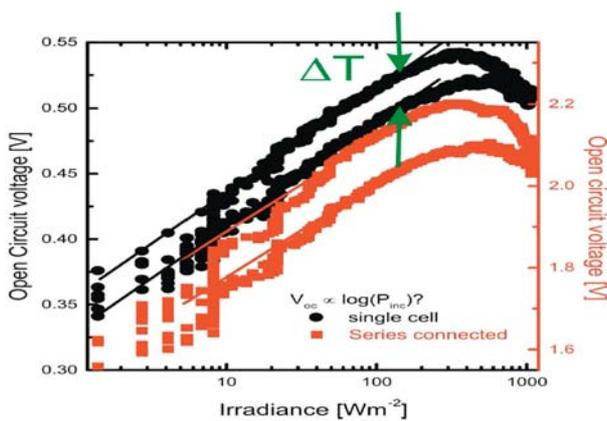
Fig. 7. Variation of  $V_{OC}$  with intensity. Temperature effects reduce  $V_{OC}$  towards high intensities.
