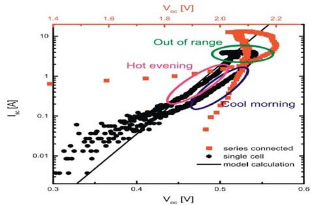
Fig. 8.  $I_{SC}$  ( $V_{OC}$ ) dependence of a single cell and a series connection of 4 cells.
