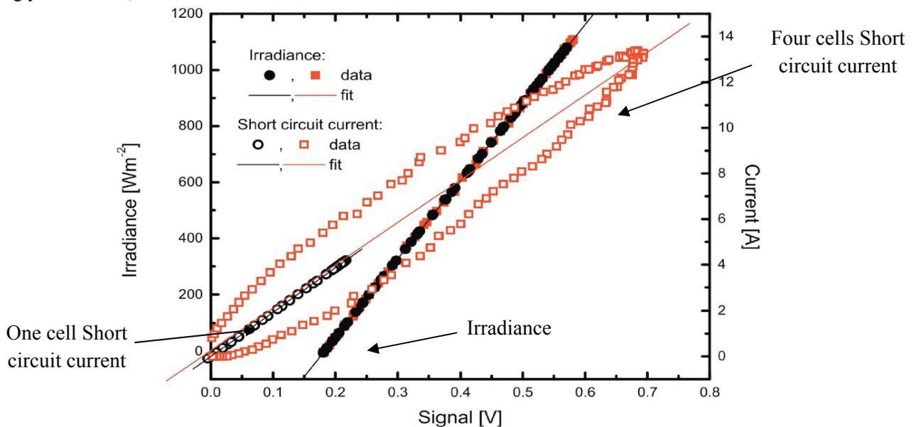
Fig. 5. Comparison between measured signal and physical units for both single and four cell arrangements.
