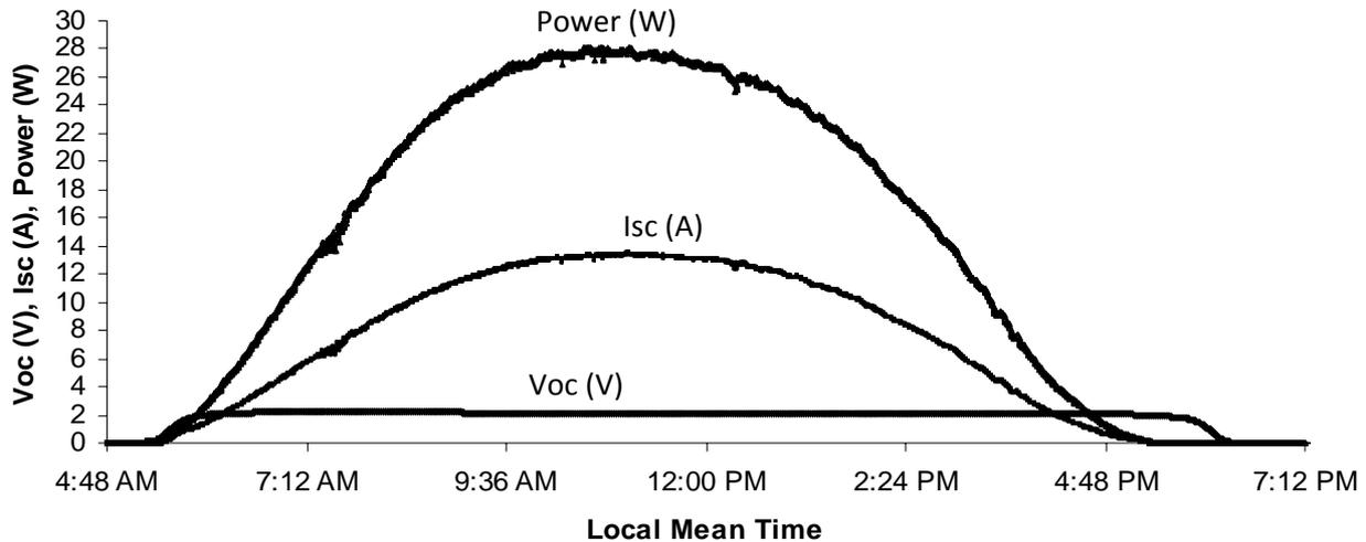
Fig. 2. Daily profile of the measured solar module short circuit current, open circuit voltage and output electrical power.
