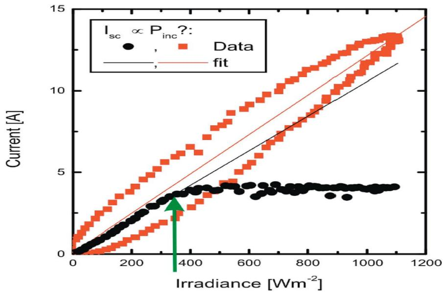
Fig. 6. Short circuit current as a function of intensity.
