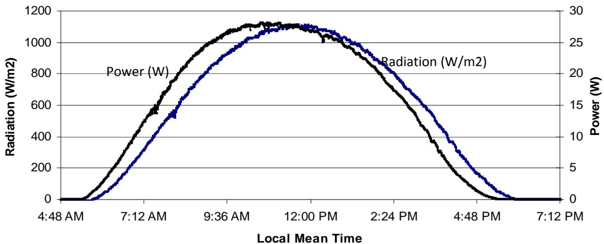
Fig. 3. Daily profile of incident solar radiation along with module output power.
