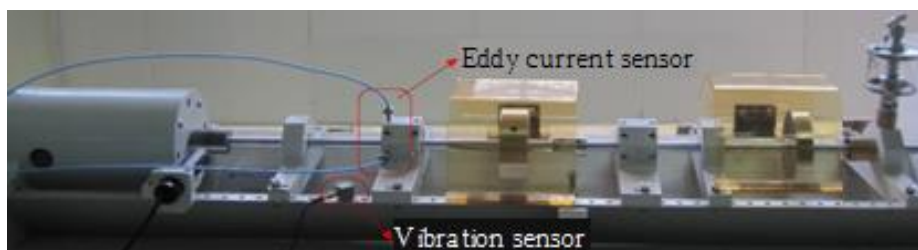
Fig. 4. Hydraulic unit vibration test bench.
