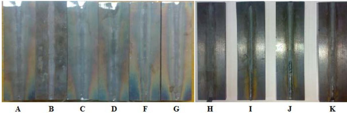
Fig. 2 Thermally influenced areas (backside of the test pieces)
