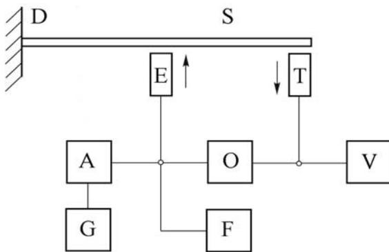
Fig. 7 The plan of the system of measurement of the sizes necessary to determine the logarithmic decrement, from the analysis of the resonance curves.
