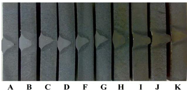
Fig. 4 The macrostructure of the belts realized with various welding statuses.
