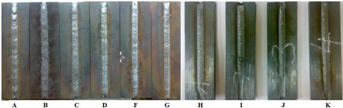
Fig. 3 The aspect of the belts realized with various welding-vibration statuses
