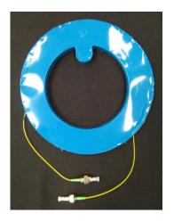
Fig. 2. Proposed interferometric measuring probe
